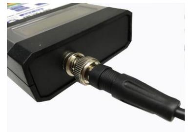
*BNC Input for Accelerometer*
